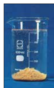
Fig. 6 Clear water with flocculated matter
